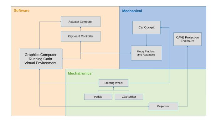
The final design of the system is categorized into three sectors: mechanical, mechatronics, and software. Each category overlaps and interfaces with each other category.
