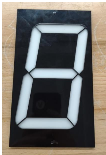
Fig. 2.10.1. Single acrylic digit prototype
