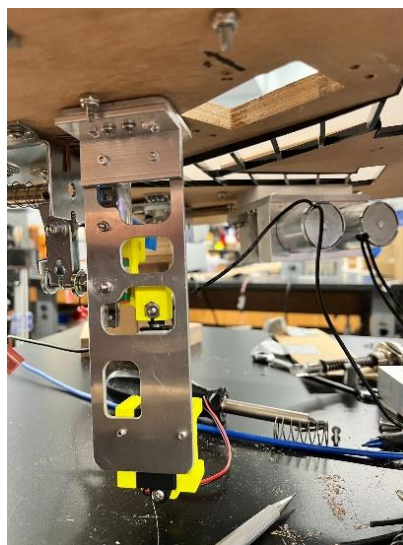
Fig. 2.7.10. Final bollard post prototype screwed into playfield
