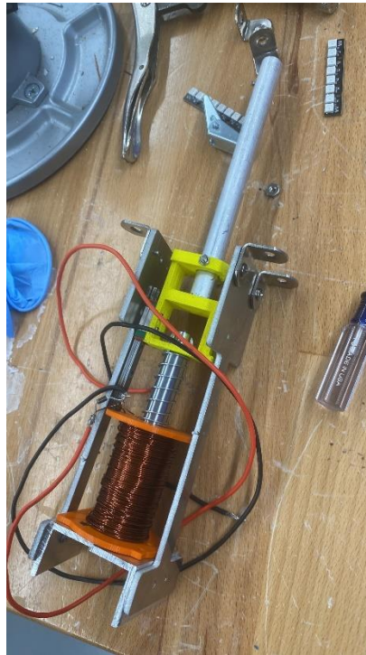
Fig. 2.3.6. Second iteration of pop bumper (pre-mounting)
