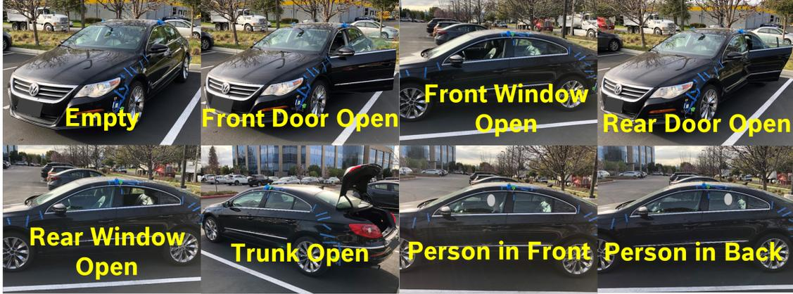
Figure 6.16: *CaraoKey* attempts to distinguish 8 car states – empty, front and rear door open, front and rear window open, trunk open, and a person in the front or the rear of the car.
