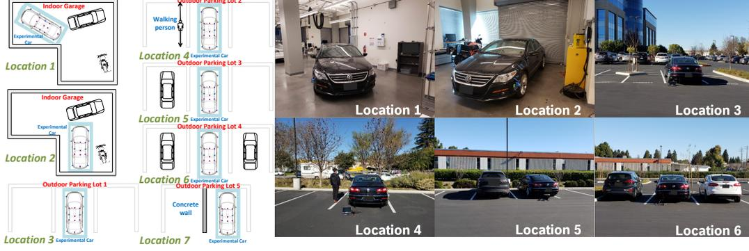
Figure 6.17: Experimental locations and scenarios: We evaluate *CaraoKey* at 7 different locations (two indoors and five outdoors), under various scenarios. Locations 1 and 2 are different indoor environments of varying multipath, in Location 3 the car is parked in free space, in Location 4 there is a person walking on the side, in Locations 5 and 6 car(s) are parked on one and both side(s) respectively, and in Location 7, the car is parked next to a concrete wall.
