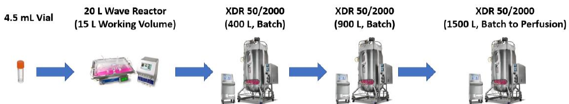
Figure 4.3. Scale-up process equipment and requirements from 4.5 mL vial to 1500 L XDR 50/2000 perfusion reactor (GE Healthcare, 2018c).
