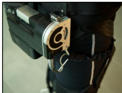
Fig 3. Bowden cable mechanism [10]
