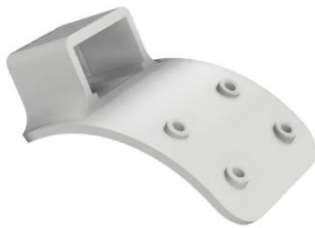
Fig 24. Improved wrist mount CAD design
