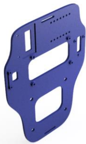
Fig 23. Improved electronic back mount CAD design
