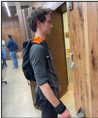
Fig 13. First prototype design displaying backpack, cable, shoulder mount, and wrist cuff
