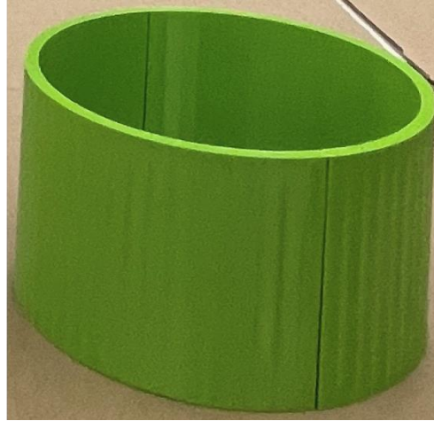
Figure 55. Extended nosecone mold (Height 10 cm)
