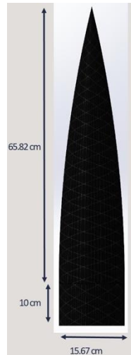
Figure 3. Final ogive nosecone design and dimensions.
