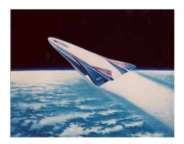
*Note*. The Rockwell X-30 depicted above was a technology demonstrator for a single-stage-to-orbit spacecraft. The program was terminated in 1993 after 7 years of development amid budget cuts and technical issues, however research on advanced materials and hypersonic flight was completed.
