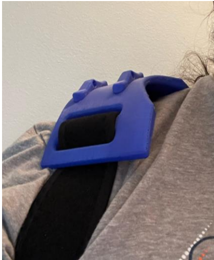
Figure 14: Neck Brace V1 Incorrectly seated on the shoulder due to strap
