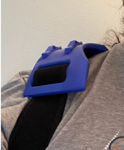
Figure 15: Neck Brace V1 Incorrectly seated on the shoulder due to strap
