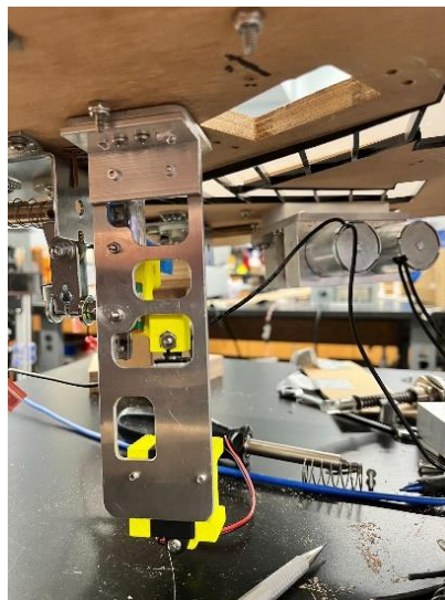
Fig. 2.7.10. Final bollard post prototype screwed into playfield
