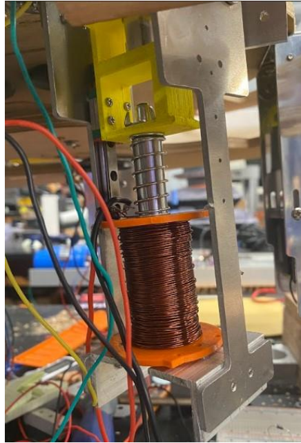
Fig. 2.3.7. Second iteration of the pop bumper mounted (below playfield view)
