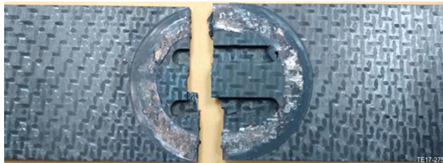
Figure 95. Stressed permeability coupon no. 7 after failure at 53.2 hours.
