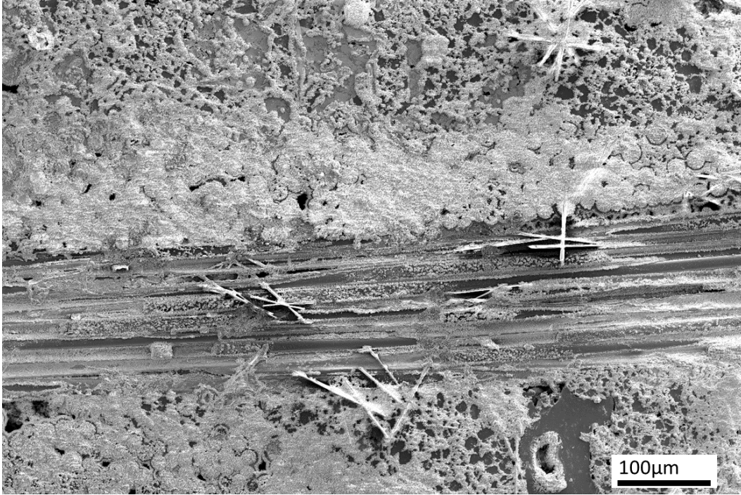
Figure 118. B-N-F deposit across the surface of a CMC (oxidized in dry O 2 , 800C, 1h) after 1h of 25 vol% HF/ 75 vol% H 2 O digestion (digestion step 3, Table 43).
