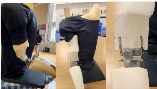
Fig. 5. Final prototype of joint reduction trainer. Final printed and cast elbow joint mechanism mounted to the shoulder and torso on a stand.
