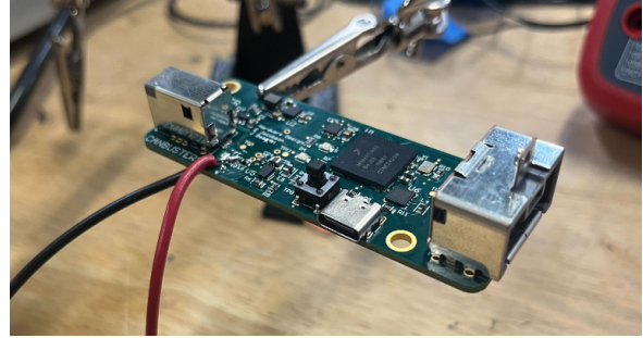
Fig. 17: Power on sequence test setup
