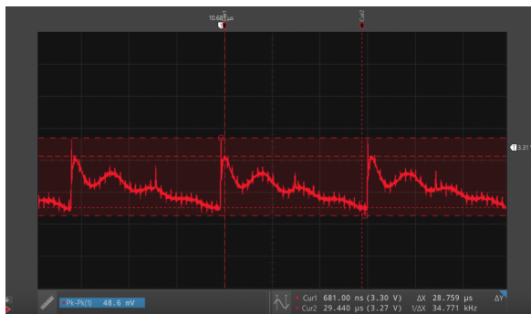
Fig. 19: 50mV pkpk DCDC ripple voltage
