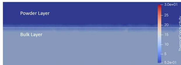
Figure 45: Initial thermal conductivity distribution between powder and substrate (longitudinal view).
