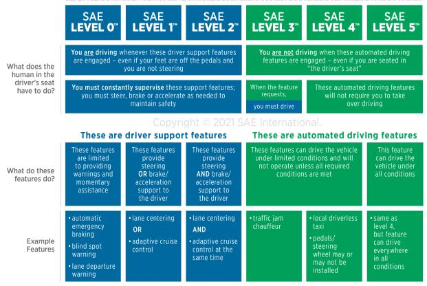
Figure 1. SAE Level descriptions and classifications for driving automation.
