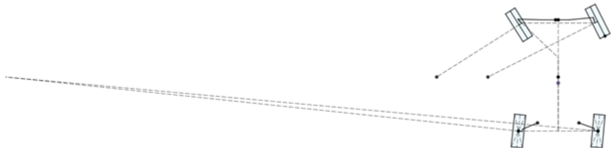
Figure 8: Virginia Motorsports' FSAE car's low speed negative rear wheel steering with 100% Ackerman rear geometry.
