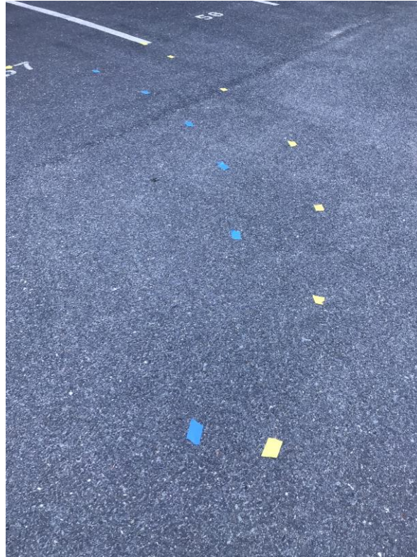
Figure 44: Close up view showing vehicle path with rear wheel steering activated (blue) and without RWS activated (yellow).
