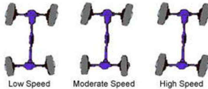
Figure 7: Speed dependent rear wheel steering (General Motors QuadraSteer Technology, n.d.).
