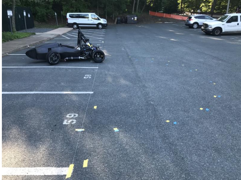
Figure 43: Turning radius test with rear wheel steering (blue tape marks path with rear wheel steering engaged). (2.89 m turning radius)
