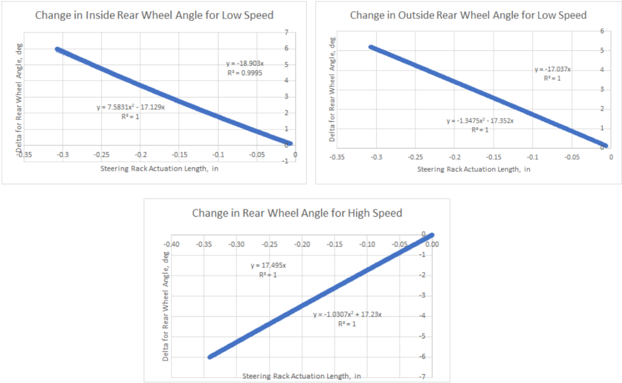
Figure 27: Delta of Rear Wheel Angle vs Actuation of Steering Rack for left and right rear wheels at low speed and high speeds.
