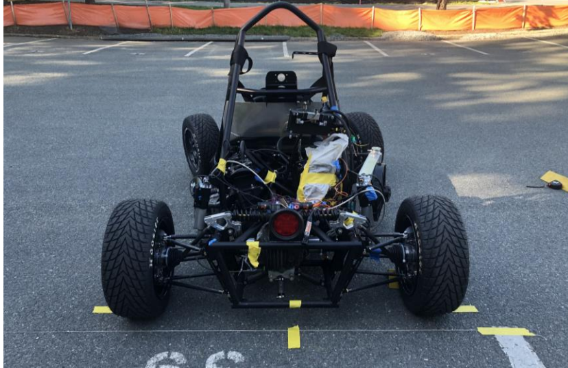
Figure 41: Turning radius test starting setup.
