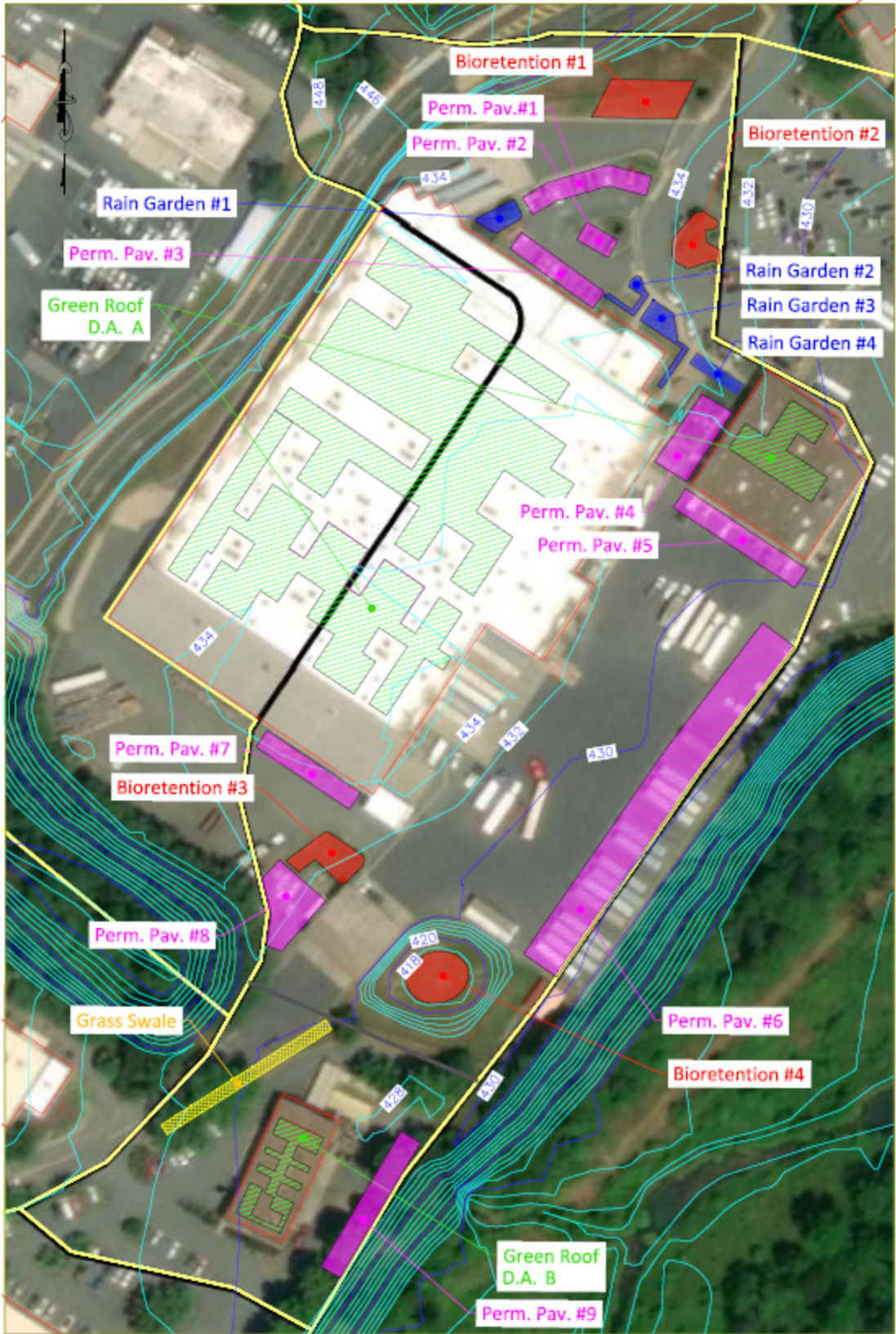
Figure 18. Plan view of site-scale design for subbasin 73571.
