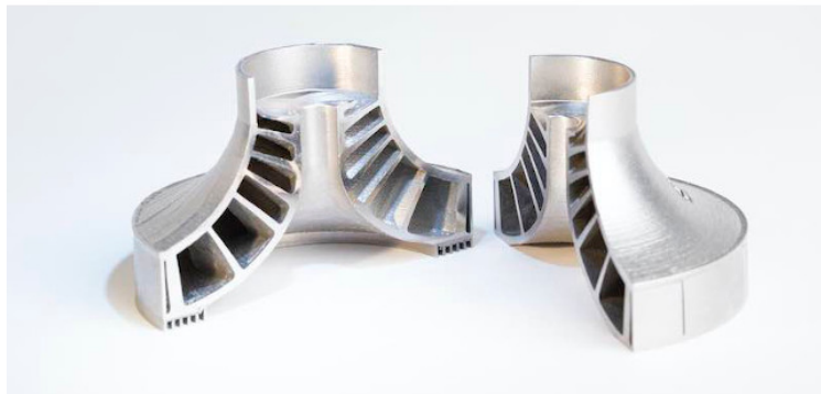
Figure 27: An additively manufactured component's complex cross section [6]
