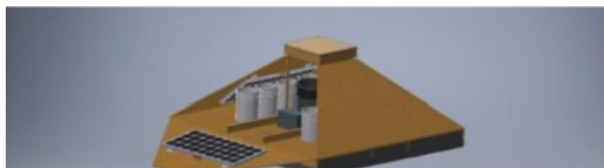
Figure 1. Note. Floating platform AutoCAD model, partially folded: An overview of the current system depicting one of the trapezoidal panels unfolded. From Hydroponic crop cultivation as a strategy for reducing food insecurity (p. 3), by Boland et al., 2022
