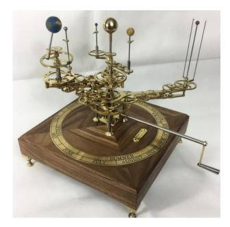
*Note.* This is a complex example of an orrery of the solar system. Notice the complexity of the gears to capture the motion of the selected planets around the sun with a constant input from the user. From *Staines & Son Orrery Makers Personal Gallery*.
