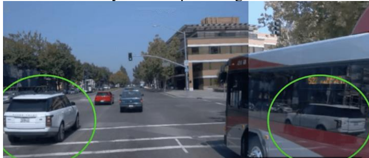
Figure 1: An edge-case scenario where the reflection of an SUV off an adjacent bus may cause perception difficulties (Adapted from Arnoud, 2018).
