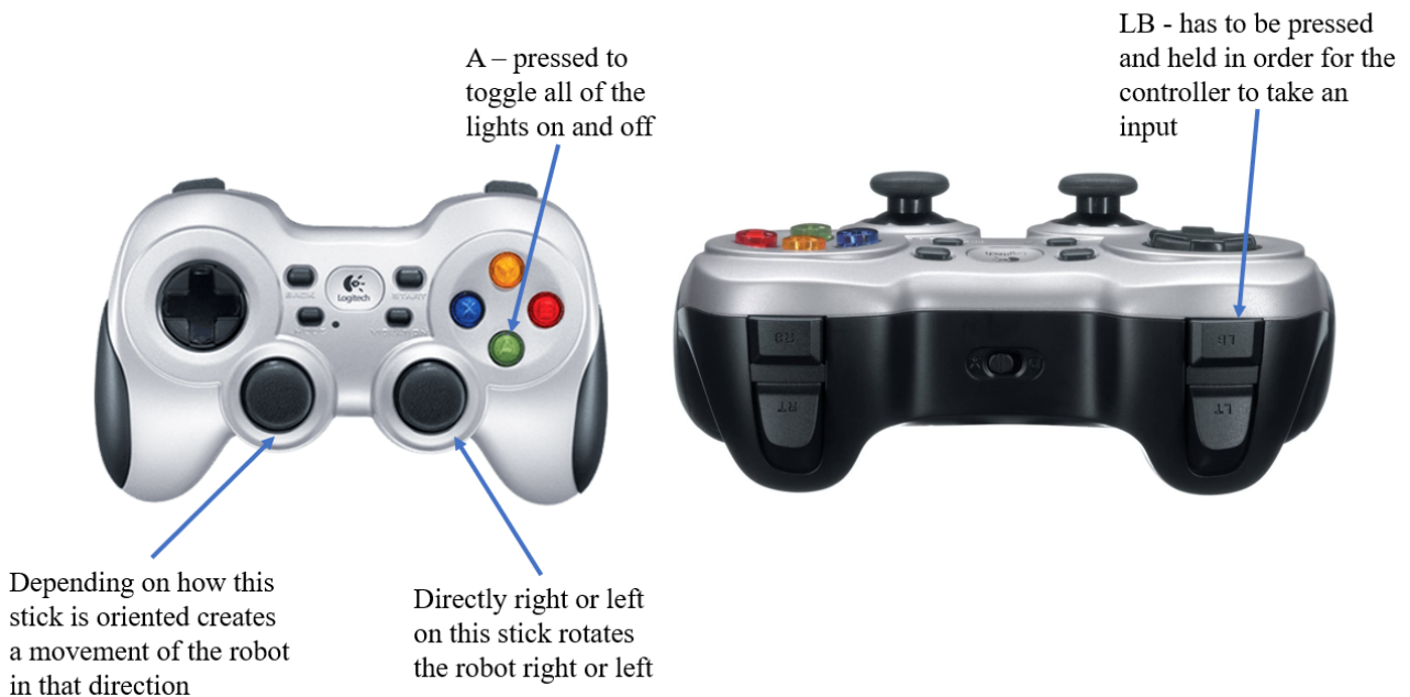
Figure 13. Control scheme for ROSIE
