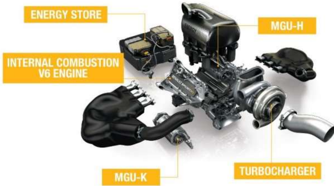
Figure 1. Formula One Hybrid Power Unit. As of 2014, Formula One racecars are powered by 1.6-liter turbocharged V6 hybrid power units with integrated energy recover units. This figure is an example of an F1 hybrid power unit with a Motor Generator Unit – Heat (MGU-H) and a Motor Generator Unit – Kinetic (MGU-K) as the methods of energy recovery. (Cassey, 2015)
