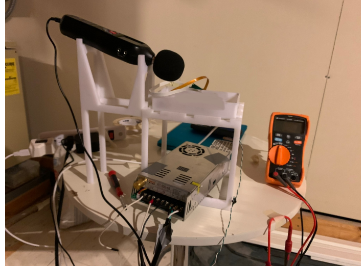
Fig. 8. Setup for noise and force testing using the decibel meter, multimeter and 12 V power source.
