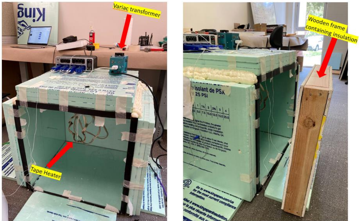
Figures 5 & 6. Above shown is the model with the locations of the Variac, tape heater, and wooden frame for the test wall labeled.
