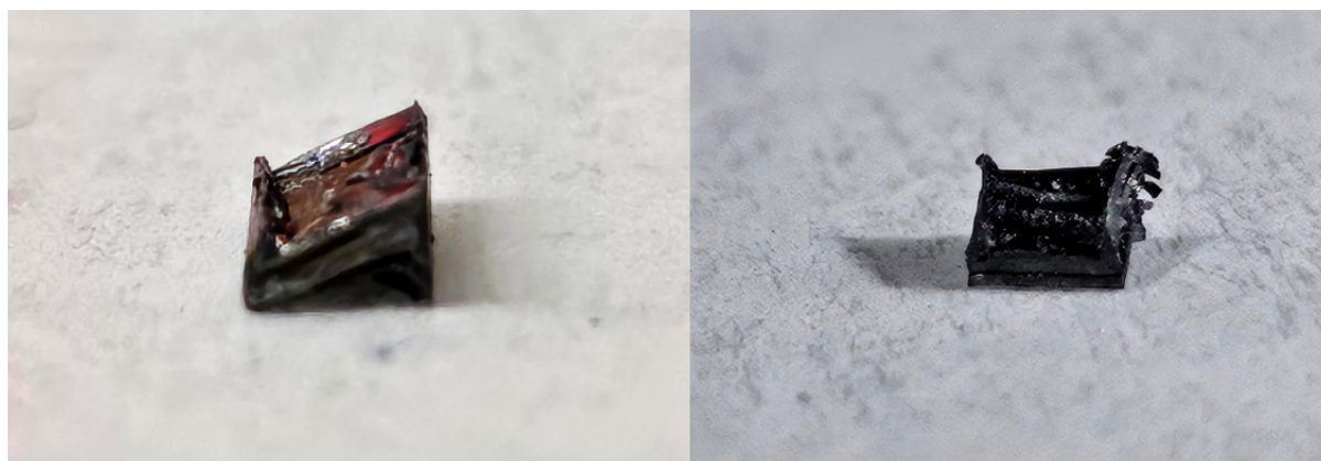
Figure 5.2: Buckled MoTe 2 crystals after application of uniaxial pressure along a or b directions. The buckling took place before a pressure of 1 MPa was applied.
