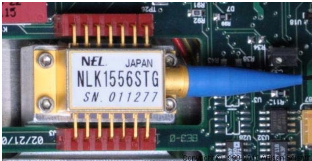
Figure 1. Picture of DFB laser diode. Model number: NEL model NLK 1556STG, 15mW output power, 14 pin butterfly, +/-1nm accuracy, PANDA-PMF fiber, FC/Angled PC connector.
