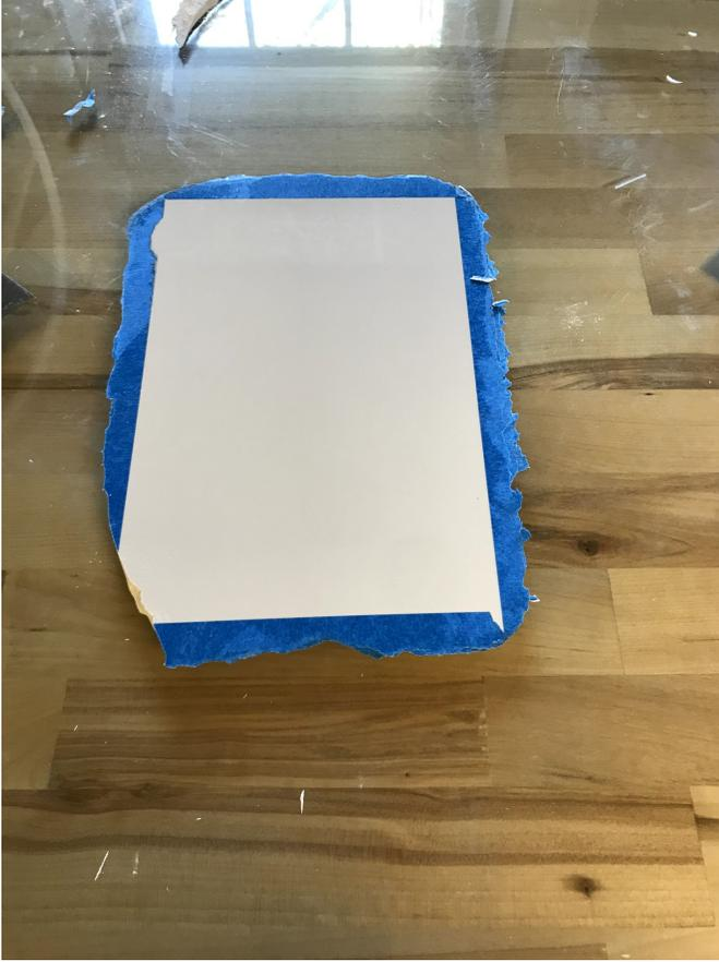
**Fig. 4.** This is the side of the -325 mesh alumina sample that was touching the glass during the infusion. It's much smoother than the top side (shown in Figure 5) because it was touching the flat tempered glass.
