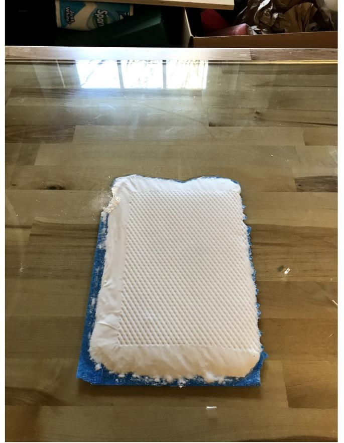
**Fig. 5.** This is the top side of the -325 tabular alumina sample. It's rougher than the smooth side because peel ply and flow media were on top of the powder before the infusion. This resulted in the pattern on the surface. For our sample disc, we smoothed this surface.
