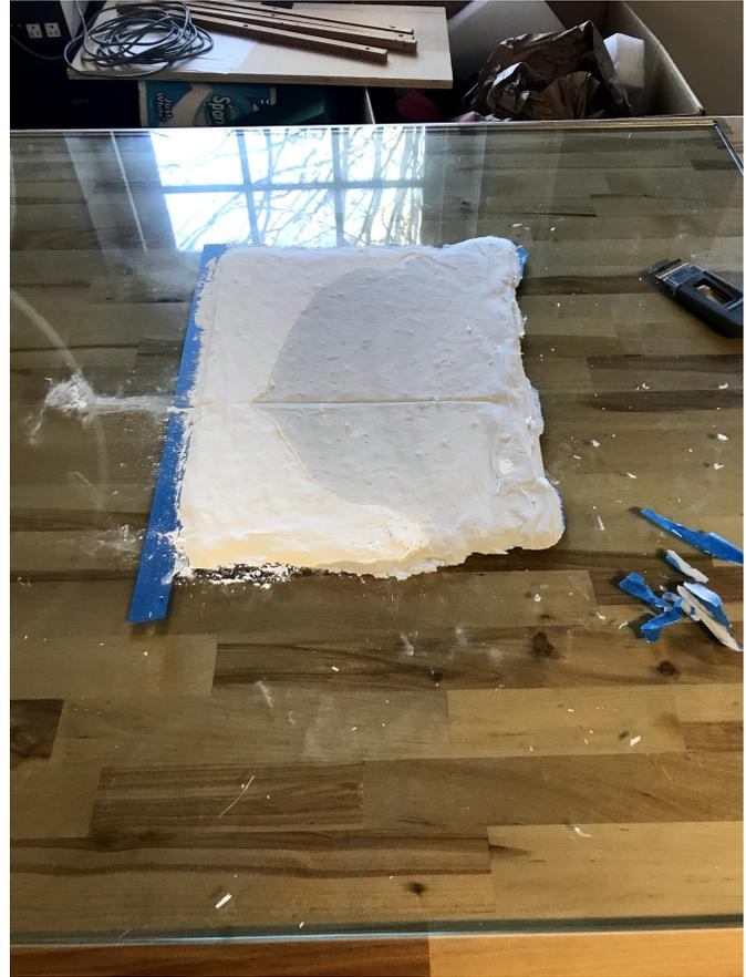
**Fig. 3.** This is an example of what happens if no flow media is used on an infusion material that is not permeable enough. Here, we performed a resin dump to try and force the infusion, rather than letting the vacuum suck the resin through the material. For clarity, a resin dump is performed by raising the bucket of resin above the infusion surface.
