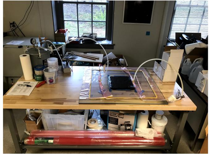
**Fig. 1.** This is an example of a finished vacuum infusion process set-up without a flow media.
