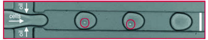
Figure 2: A real-time annotated image of a t-junction microfluidic device encapsulating cells. The gel and cell solution flows down the top channel. It meets at the “t junction” where two oil channels meet. This pinches off the gel solution, encapsulating cells in the gel. Adjusting the flow rates can lead to single cell encapsulation or cell clustering. This is the main microfluidic design for the experiments in this project.
