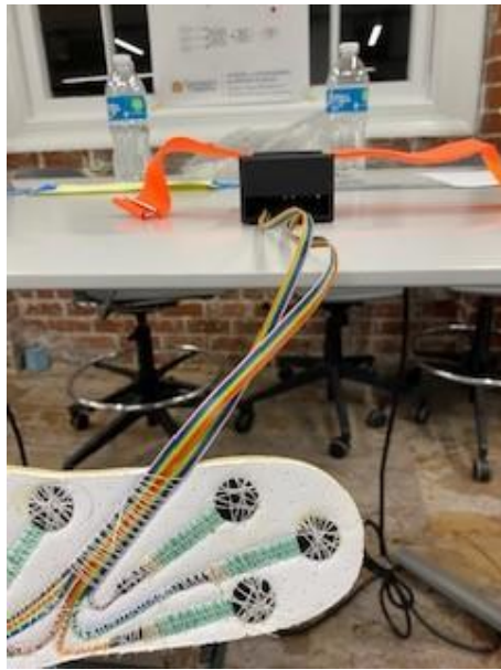
Figure 35: Shoe Sole Sensor Placement
