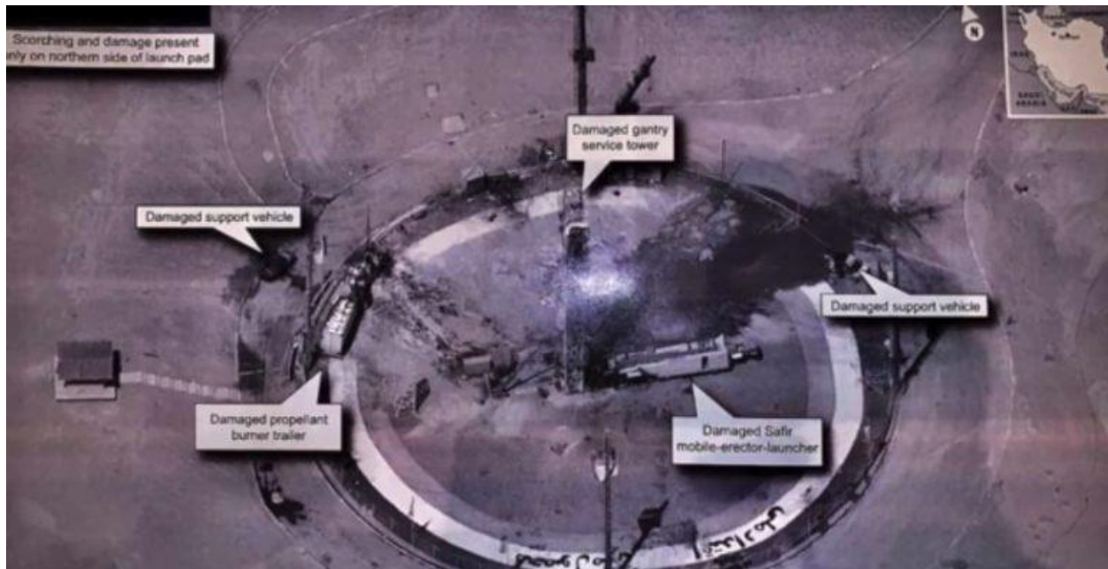
Figure 1: Satellite imagery with a resolution of 10cm of a failed Iran satellite launch
