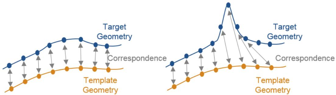
Figure 19 difficulty in finding corresponding points between target and template geometries
