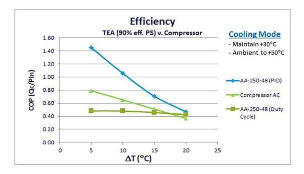
Efficiency of Thermoelectric and Compressor Coolers at Different Temperature Differentials
