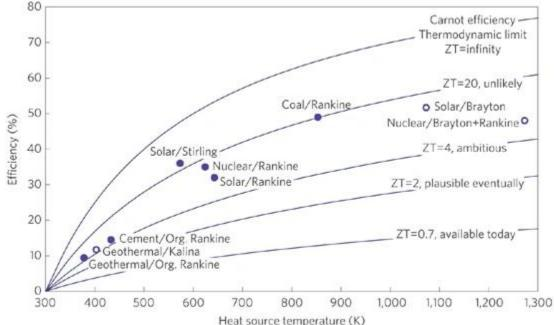
Required efficiency for Thermoelectric materials to generate electricity to compare with existing
