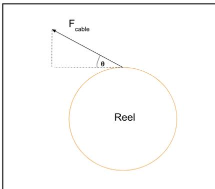
Fig. 7 Diagram depicting how cables will be acting at an angle to the reel that houses the motors. The horizontal component of the force induces a torque about the center.
