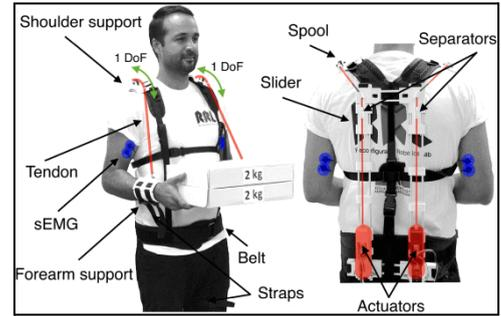
Fig. 3 Reconfigurable Robotics Lab, SEMG-Driven Soft ExoSuit
