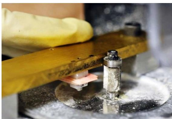
Figure 2.5 Cortical Bone wafers being milled.
