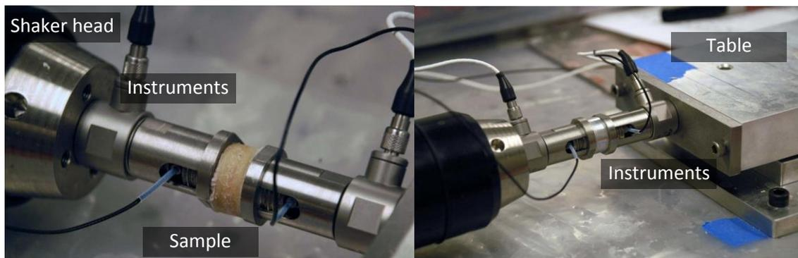
**Figure 6.1 Transmissibility Test setup; Shaker and shaker-side instruments (left); Index table and table-side instruments (right); please note that an aluminum placeholder sample is installed in the image on right.**
