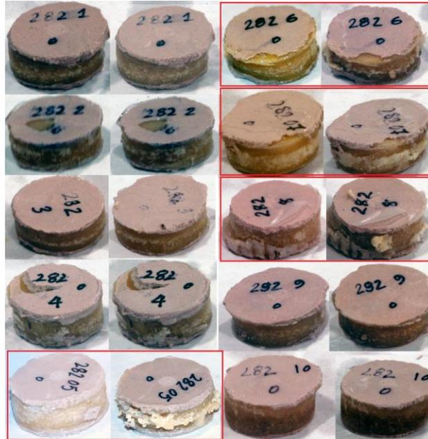
Figure 5.7 Calvarium core samples, belonging to subject 3, before (columns 1 and 3) and after (columns 2 and 4) testing. Failure cases have been shown by the red boxes.
