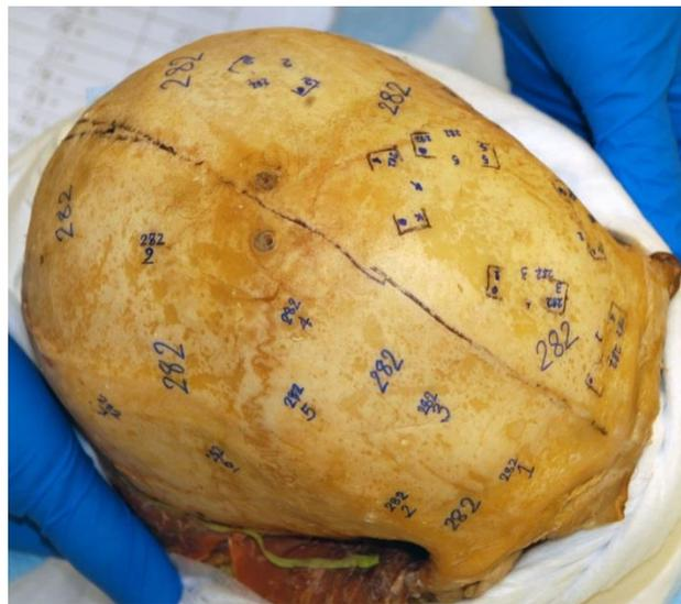
**Figure 2.1 Sample harvest locations marked on the calvarium; through-the-thickness cylindrical samples (cores) from the right half (bottom left of this image) and cortical coupon samples from the left half of the calvarium (top right of this image)**
