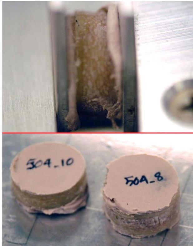
**Figure 5.1** A skull core being potted (top) for mounting on the test device and two typical potted cores (bottom).
