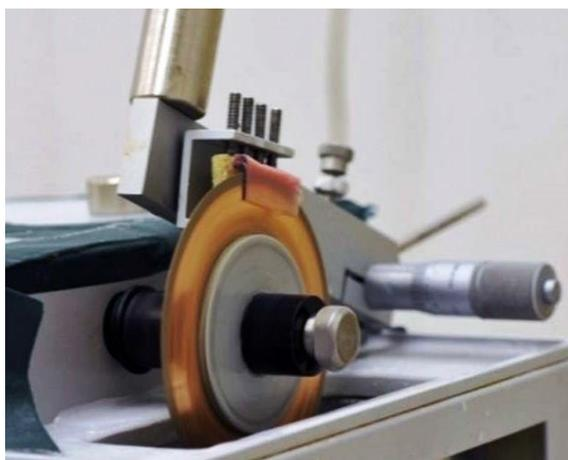
Figure 2.4 0.5 mm thick cortical bone wafer being machined on a Buehler Isomet low-speed saw.
