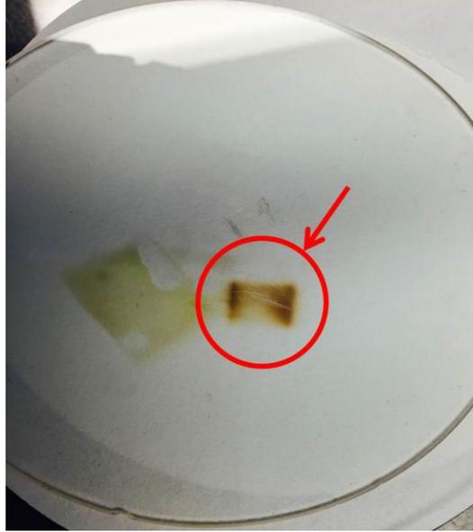
Fig. 4.2. Black material deposited on the quartz cover slide during thermal activation at 300 °C for 2 minutes. The black material in the red circle is speculated to be out-diffused sulfur.
