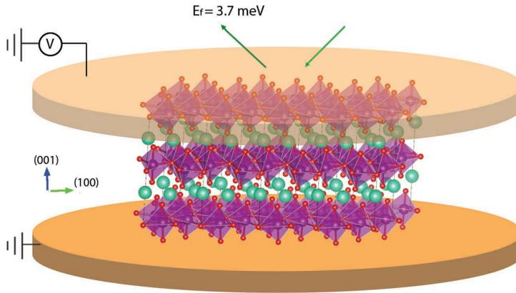
Figure 3.3 – Shown above is a schematic plot showing the experimental setup. The (001)-cut single crystal  $\text{LuMnO}_3$  sample was glued between two Al plates by silver paint. The Al plates served as parallel plate capacitor and provided static electric field across the sample.
