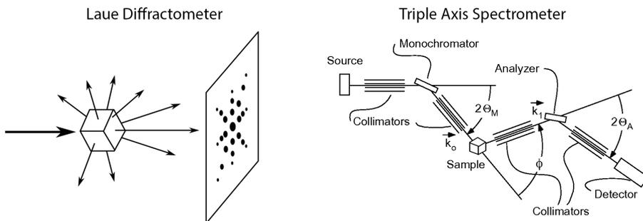
Figure 2.3 – Schematic plot of Laue diffractometer (left) and triple axis spectrometer (right). [94]
