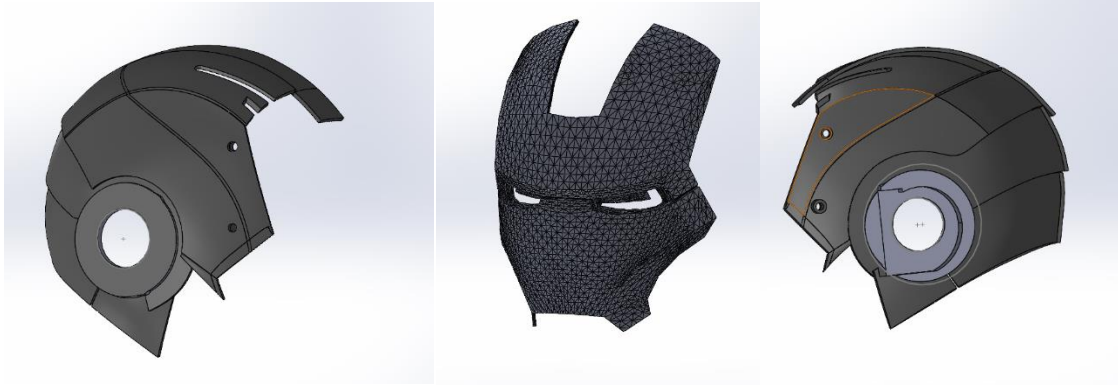
Figure 1: Initial Iron man helmet design for the Clean-19. From left to right we have the three parts of the mask: The right side of the helmet, the face mask, and the left portion of the helmet.
