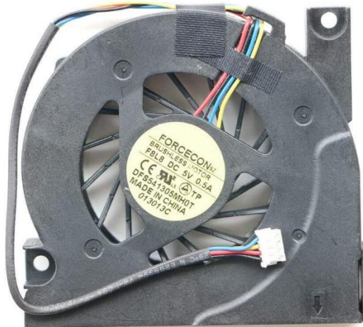
Figure 2: CAQL CPU Cooling Fan with PWM capability to be attached within the helmet.
