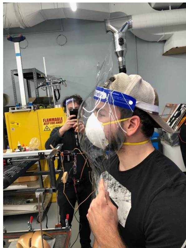
Figure 20: The face shield portion of our Iron Man helmet PAPR created from thermoformed plastic.
