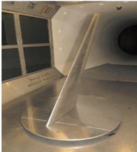
Fig. 1. 8.9% scaled CRM65 wing installed in Wichita State University's Walter H. Beech Wind Tunnel. [11]
