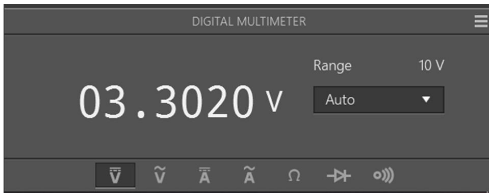
Figure 25: 3.3V Power Supply Verification (Remote)
