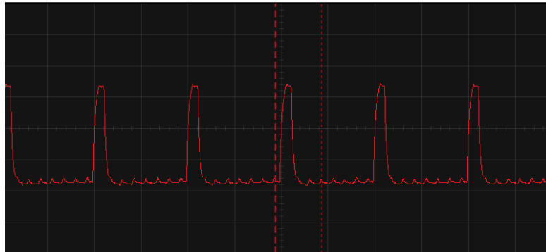
Figure 44 Servo Signal with Lowpass Filter
