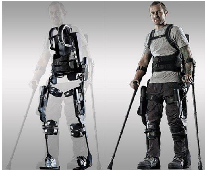
Figure 1: Exoskeleton to assist patients with “lower extremity weakness” (Genesis, 2018).
