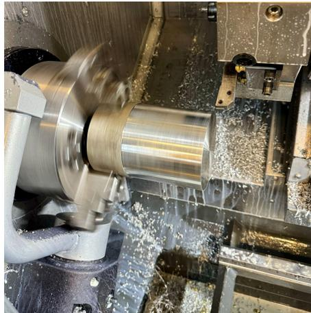
**Fig. 14:** *Haas* Lathe Setup, Three-Jaw Chuck Rotating the Aluminum Hub.
