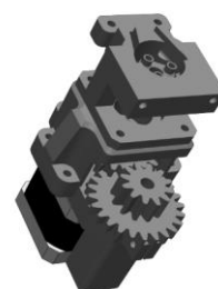
Figure 2: 3D SOLIDWORKS rendering of peristaltic pump.
