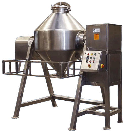
Figure 4.5.1: Double Cone Blender from ROSS
