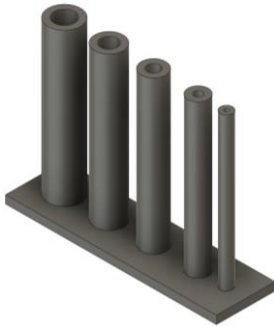
Fig. S1. Model of the hollow tubes created in Fusion, used to test the resolution of hollow printing.
