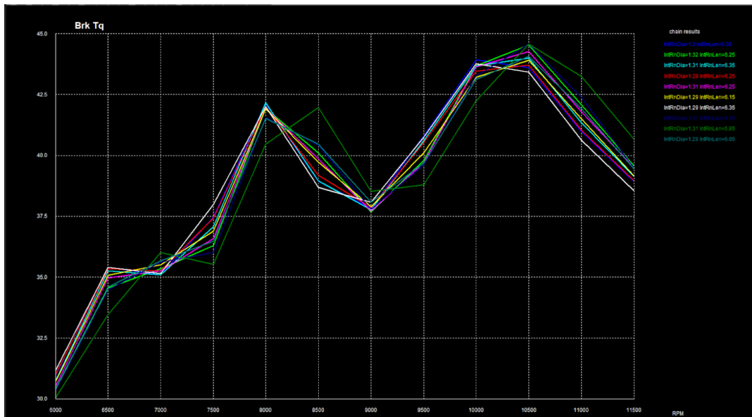
Figure 20. Preliminary Simulation, Runner Diameter and Length variation
