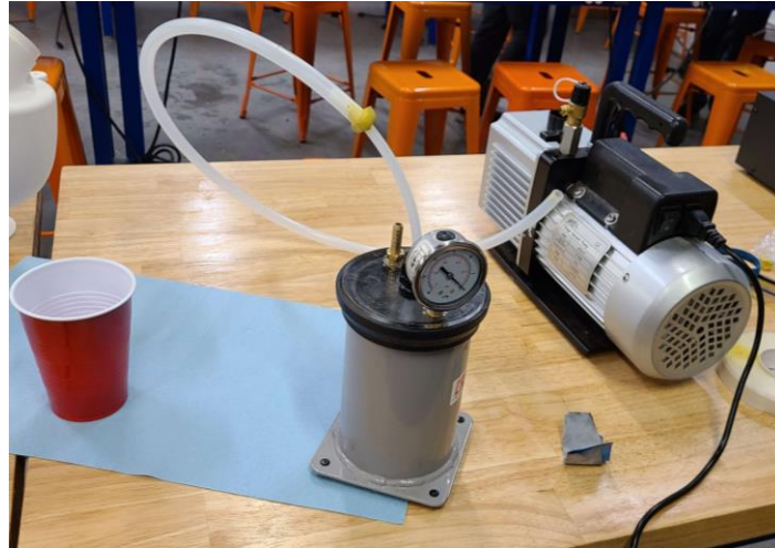
Figure 31. Vacuum Pump used to Remove Air from the Epoxy Mixture
