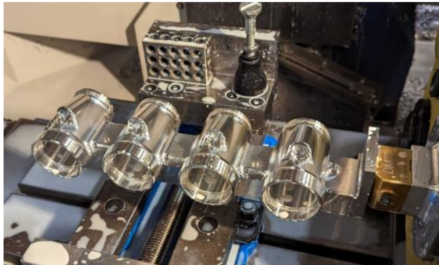
Figure 29: Semi-finished runners in 5 axis trunion.
