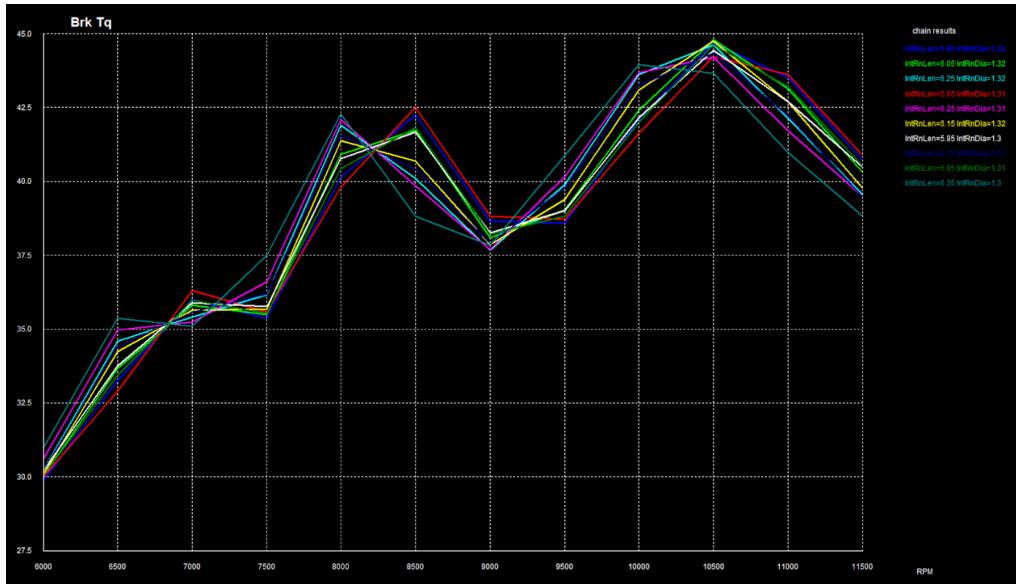
Figure 21. Refined Runner Length and Runner diameter simulation
