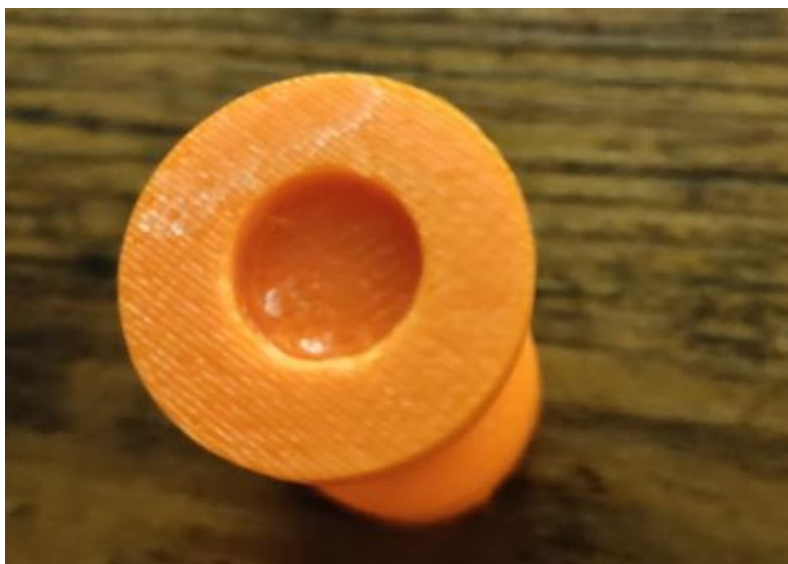
Figure 23: Chess piece with bottom cut out for magnet
