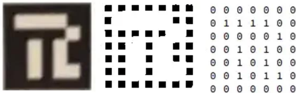
Figure 9: ArUco Marker Breakdown
