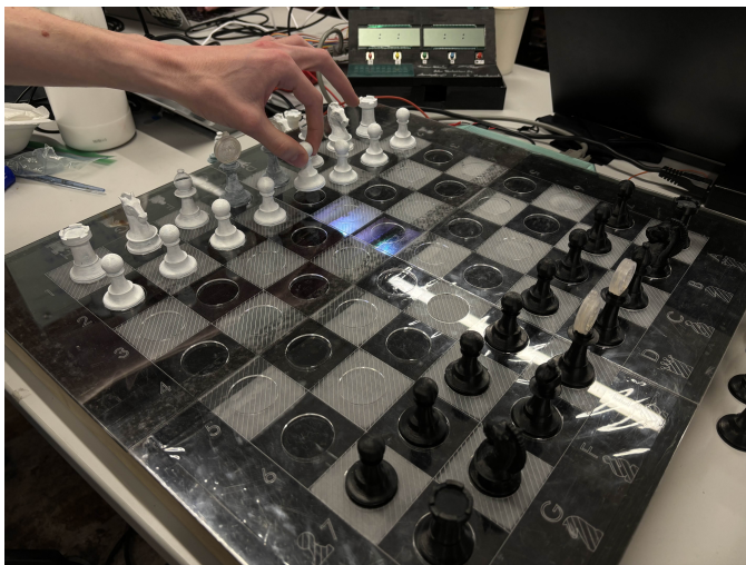
Fig. 24. The white D pawn being moved. The LEDs light to indicate which spaces are available for movement.
