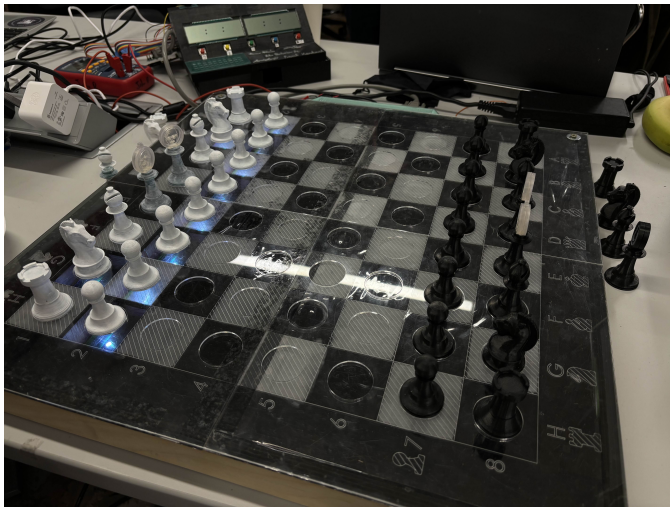
Fig. 23. The start state of the untimed board. All available moves are highlighted with the LEDs.
