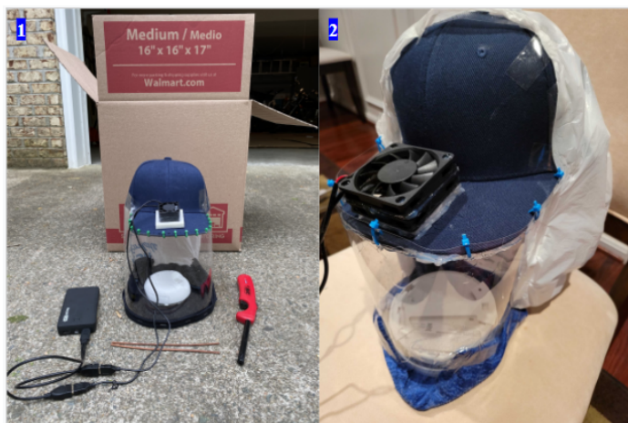
Figure 6: The smoke test materials and setup. The left image (1) is the materials used for the experiment and right image (2) shows how the back of the hat was sealed and the smoke detector was placed within the protective volume.
