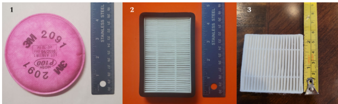
Supplementary Figure 3: The three filters: (1) 3M 2091 P100, (2) Kenmore HEPA, (3) Aurora H13 HEPA that are NOISH or equivalent certified that we chose to use in our team prototypes.
