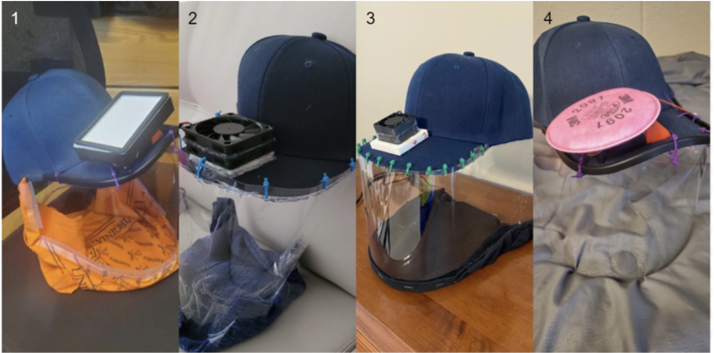
Figure 4: Four physical prototype designs that were built by each team member. (1) Model A used one 50 mm centrifugal fan mounted on bottom of the Kenmore HEPA filter, (2) Model B used two 60 mm axial fans connected in series mounted on top of the Aurora HEPA filter (3) Model C used two 40 mm axial fans connected in series mounted on top of the Aurora HEPA filter, and (4) Model D used one 50 mm centrifugal fan mounted on the bottom of the 3M 2091 HEPA filter.
